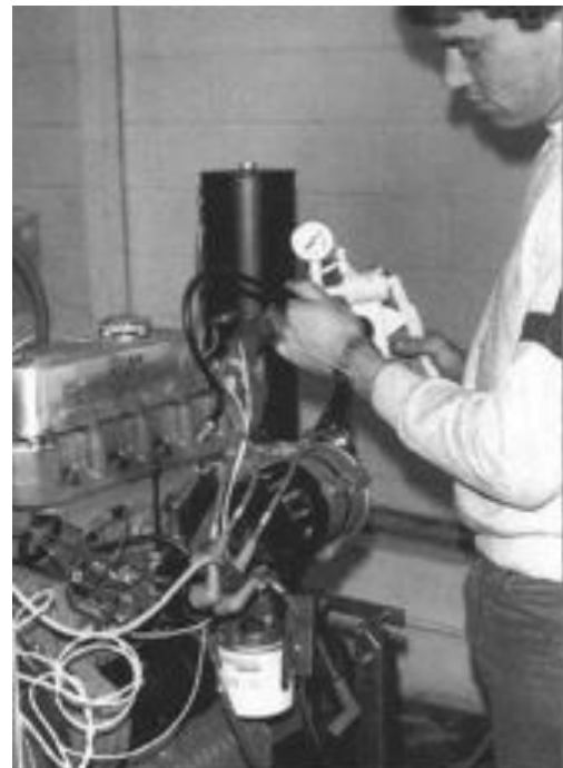
Above: After developing the cylinder-head's airflow potential, the heads must be dyno tested. On this Superflow dyno, tests are done both steady state and accelerating to establish an overall performance rating.
